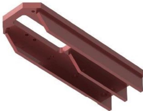
Figure 9: Rendered CAD model of the new cantilever support, bottom view
