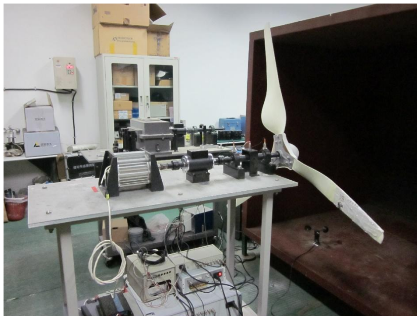
Figure 2. Test rig of direct-drive wind turbine
