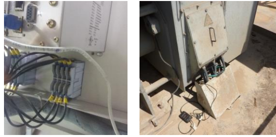
Figure 5 : measurement of Stator current and Rotor current
