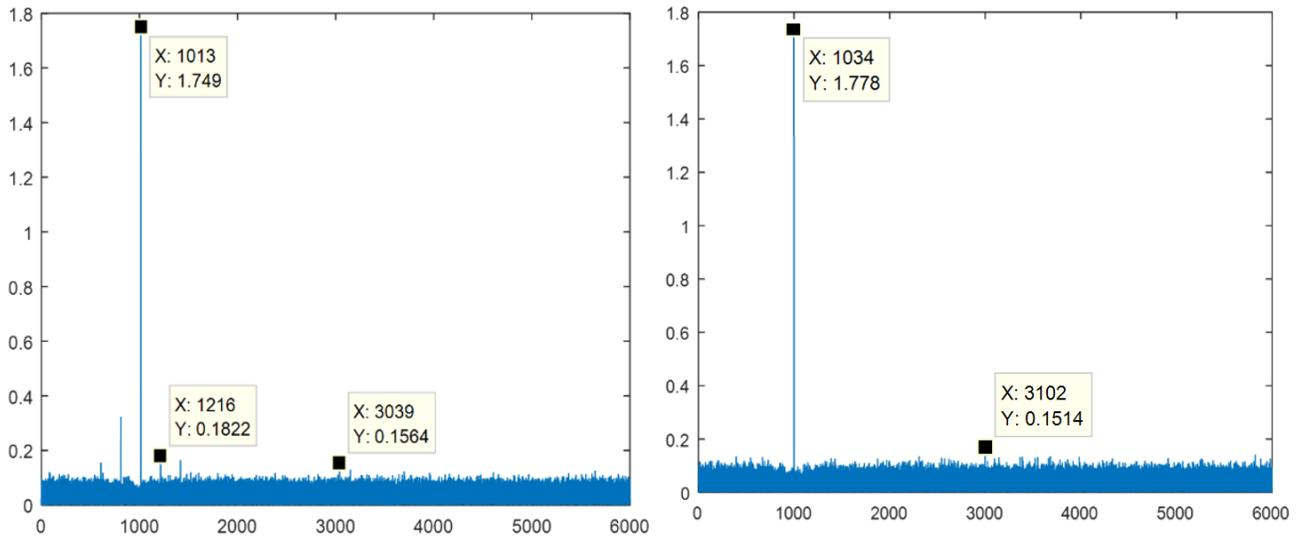
Figure 9: Comparison between two DFT of a triangular signal having a frequency of 1 kHz and sampled using a JRS (on the left) and an ARS (on the right)
