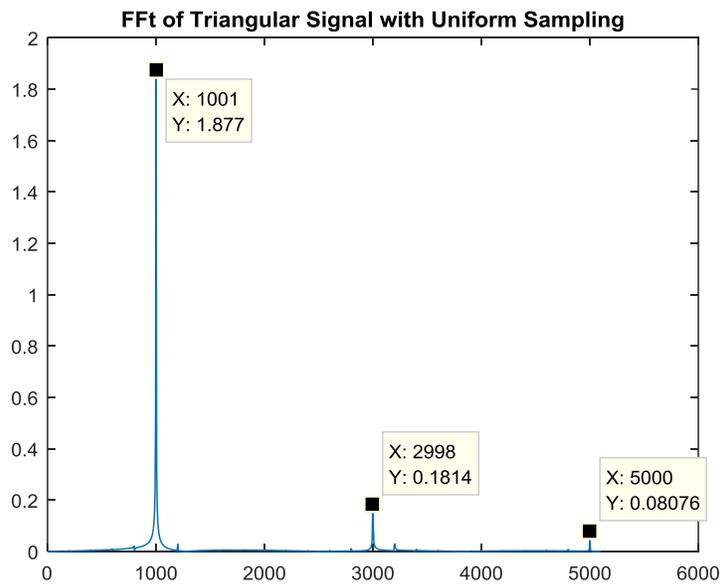
Figure 8: FFT of the Triangular Waveform with Uniform Sampling
