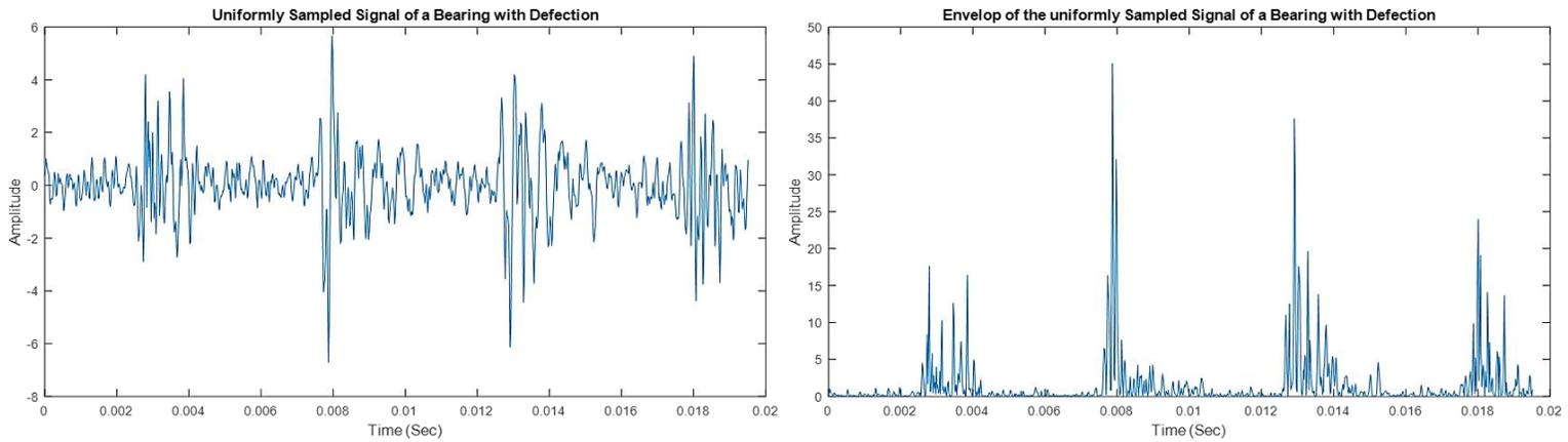
Figure 16: The Uniformly Sampled Signal of Defected Bearing Time Domain and its Envelop
