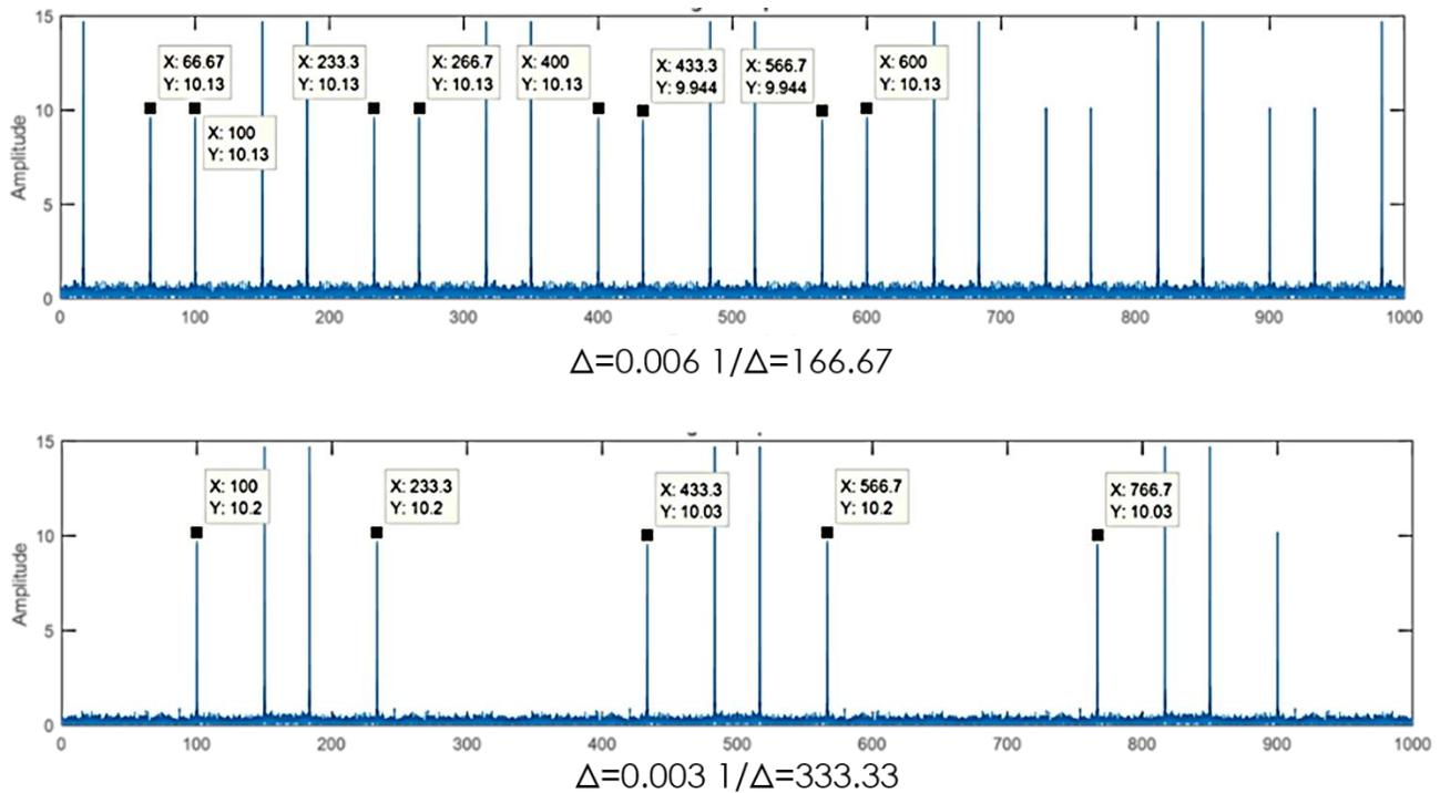
Figure 2: Two simulations of a signal having two frequencies 100 Hz and 150 Hz with applying a quantization step = 0.006 in the top and step=0.003 in the bottom.
