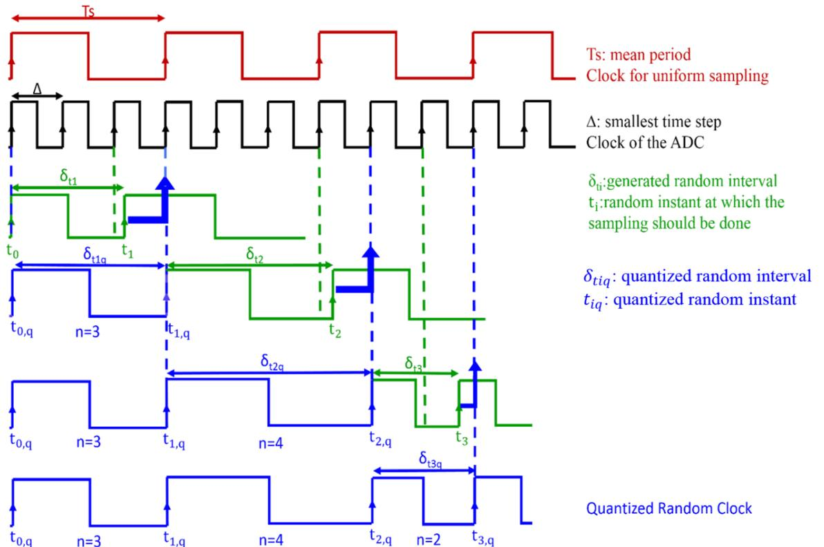
Figure 1: an example of time quantization mode for  $q_T=3$
