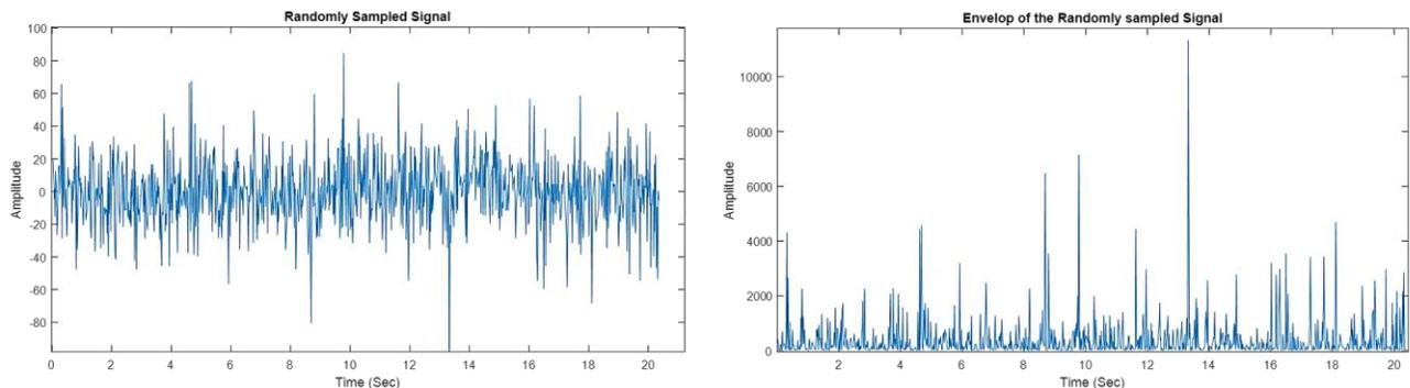
Figure 18: The Randomly Sampled Signal of the Defected Bearing and its Envelop in Time Domain
