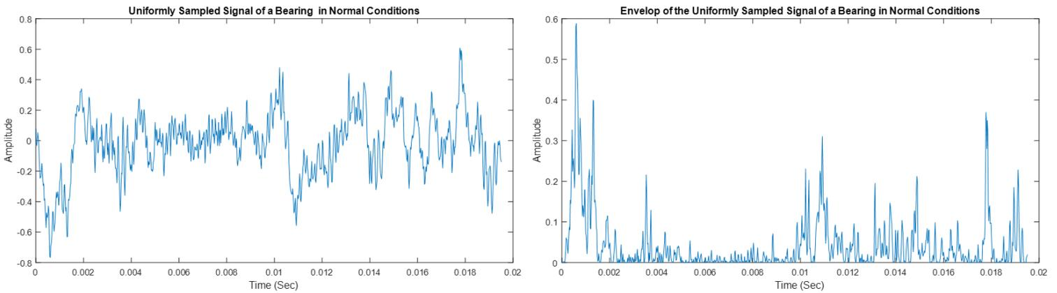
Figure 12: The Uniformly Sampled Signal of the Normal Bearing and its Envelop in Time Domain
