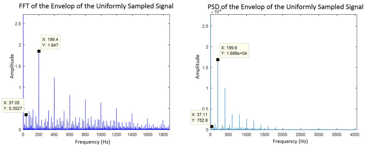
Figure 17: The FFT and the PSD of the Envelop of the Vibration of a Bearing Acquired with Uniform Sampling.
