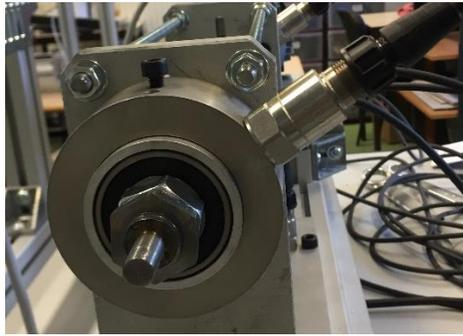
Figure 11: The Accelerometer Acquiring Vibrational Signals from the Bearing
