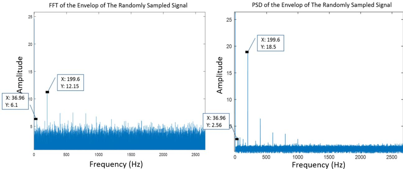
Figure 19: the FFT and the PSD of the Envelop of the Randomly Sampled Signal of the Defected Bearing using ARs with Uniform Distribution.
