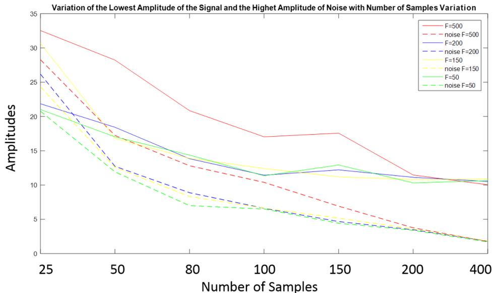
Figure 5: Comparison of the Smallest Amplitude of the Signal to the Noise in JRS with Uniform Distribution
