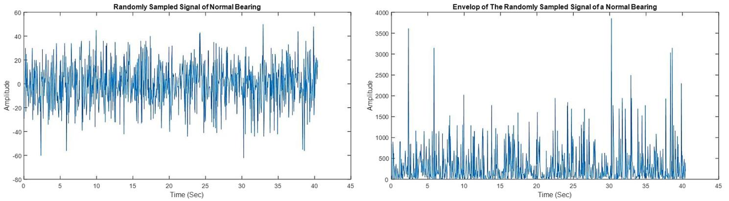
Figure 14: the Randomly Sampled Signal of the Normal Bearing and its Envelop
