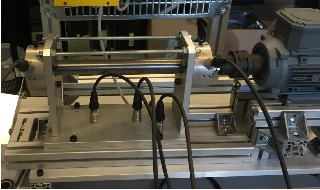
Figure 10: The Bench Containing the Rotating Motor with Bearing
