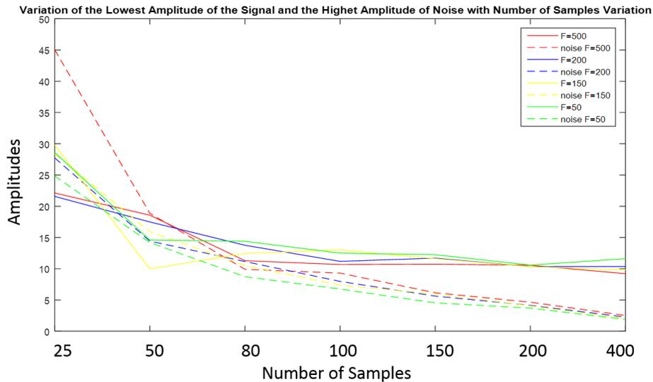
Figure 4: Comparison of the Smallest Amplitude of the Signal to the Noise in ARS with Gaussian Distribution
