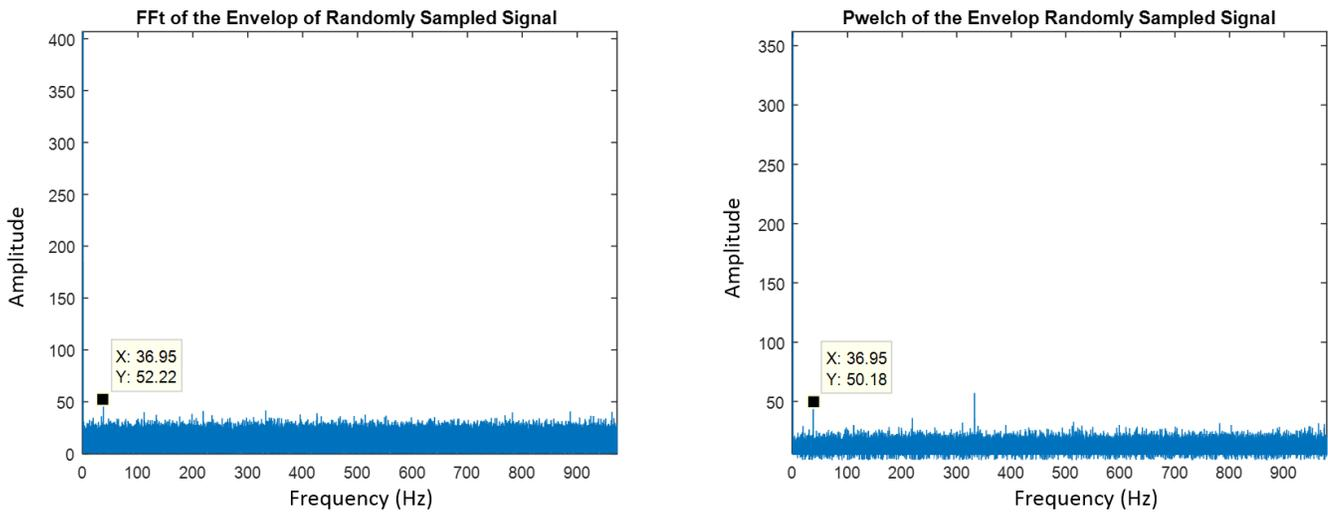
Figure 15: the FFT and the PSD of the Envelop of the Randomly Sampled Signal of the Normal Bearing
