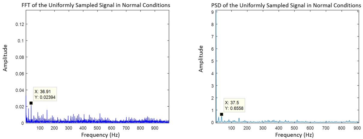
Figure 13: the FFT and the PSD of the Envelop of the Uniformly Sampled Signal of a Normal Bearing
