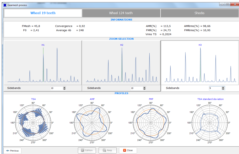
Figure 3: Analysis window of the gear processing module
