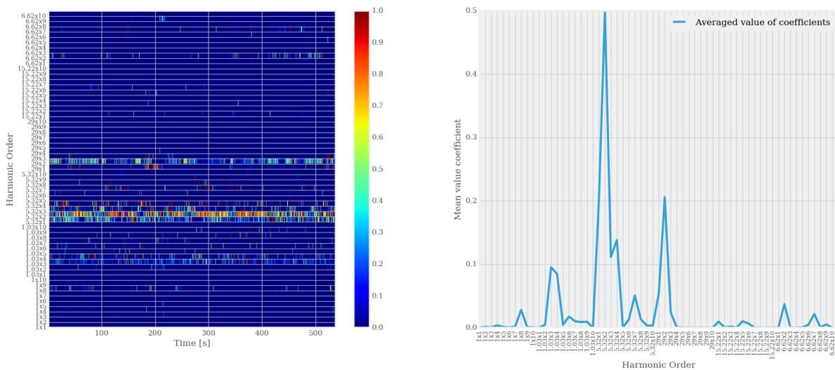
Figure 4: (a) 2D-map of the coefficient values for every harmonic order (from 1 to 10 for every fundamental order) and for every time step. (b) The time averaged coefficient values for every harmonic order.
