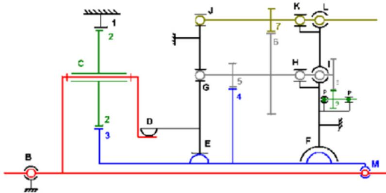
Figure 2: Visualization of the wind turbine gearbox used in the CMMNO 2014 diagnosis contest.
