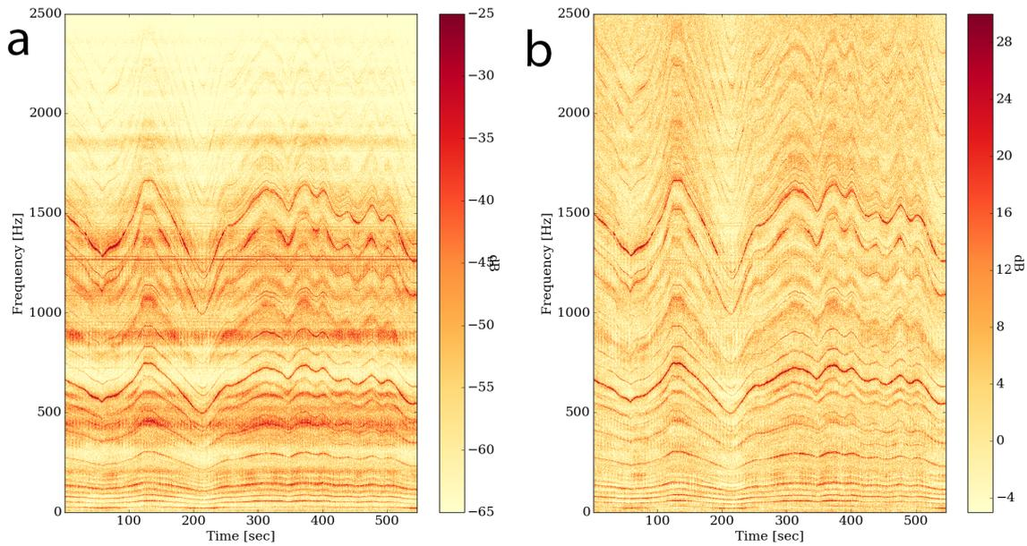
Figure 3: (a) Spectrogram of the CMMNO 2014 vibration signal of the wind turbine gearbox housing. (b) Whitened spectrogram
