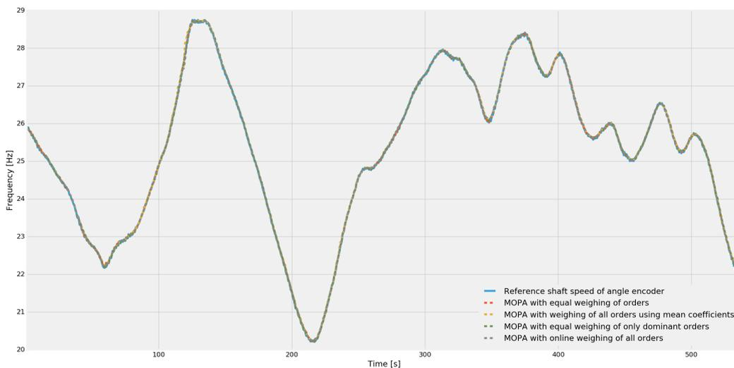
Figure 5: Shaft speed estimation results of the different weighting approaches for the MOPA method.
