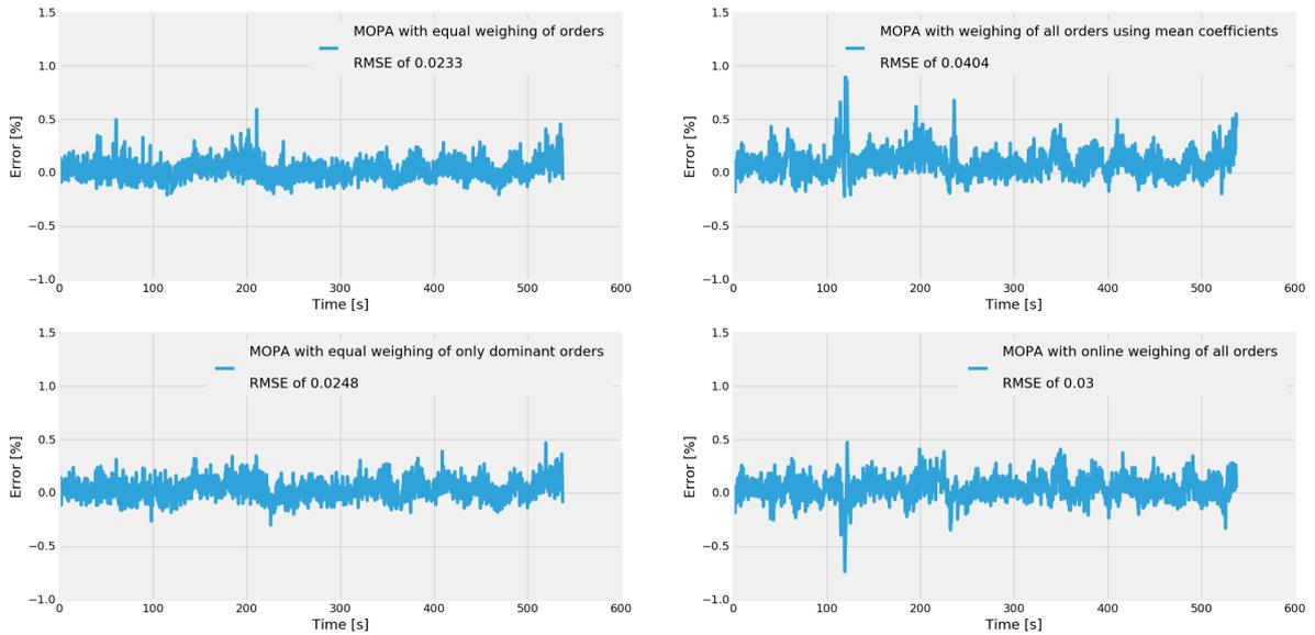
Figure 6: Relative errors between the reference shaft speed and the different approaches for the MOPA method.
