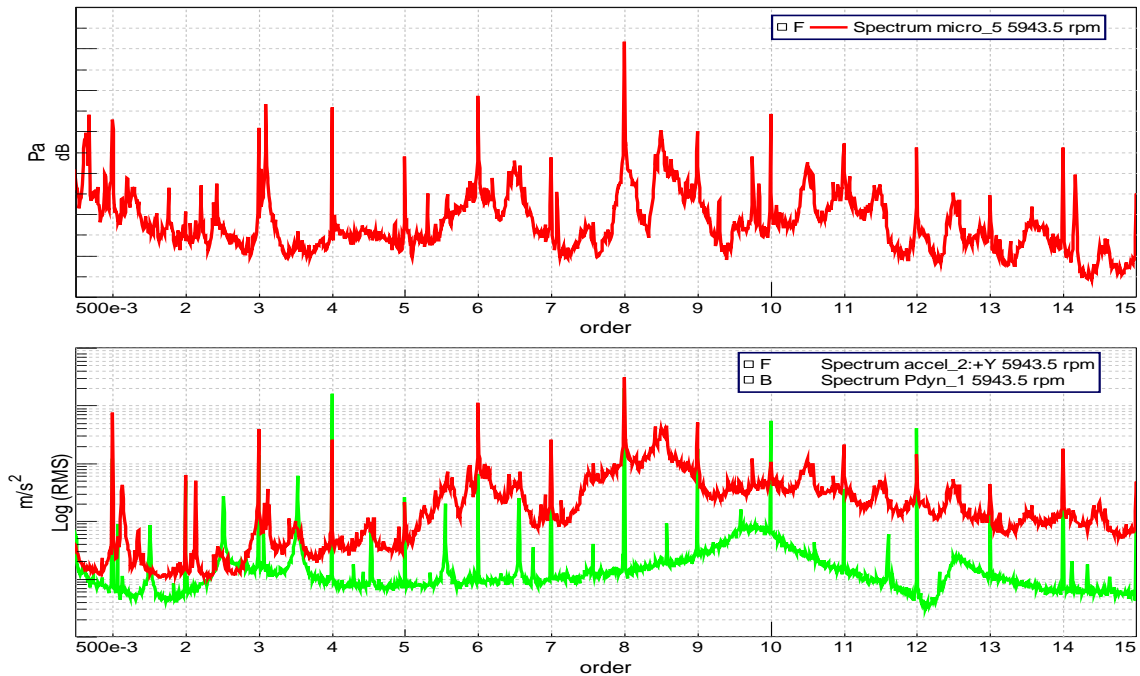
Figure 10: Order spectrum ( \Delta order = 0.01); Pump 3 Top: Microphone 5 (scale: 5 dB/div) Bottom: Gear housing accelerometer (red); dynamic pressure stage 6 (green)
