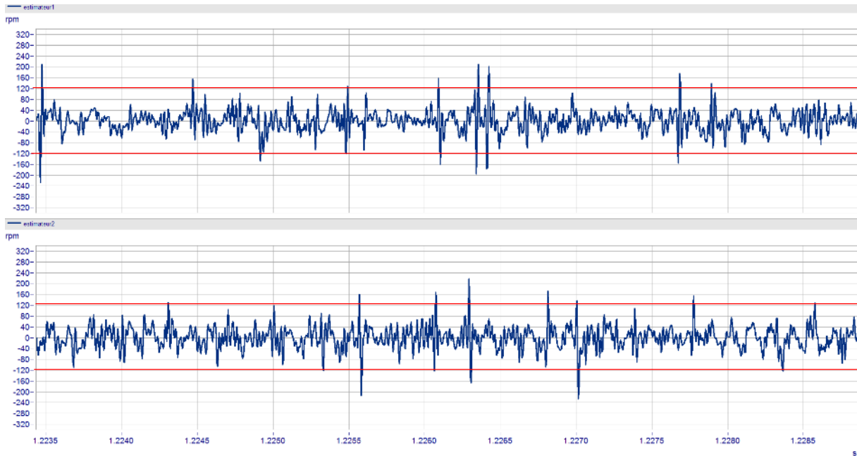
Figure 19: Relative speed signal Top: A-type response; Bottom: B-type response
