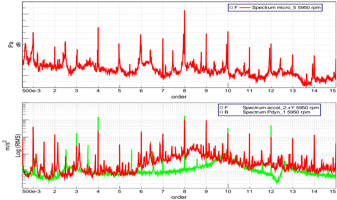
Figure 9: Order spectrum ( \Delta order = 0.01); Pump 1 Top: Microphone 5 (scale: 5 dB/div) Bottom: Gear housing accelerometer (red); dynamic pressure stage 6 (green)
