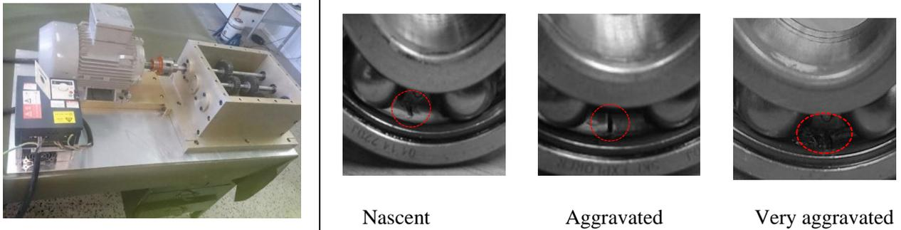
Figure 1: Test Bench & Simulated Bearing Defects
